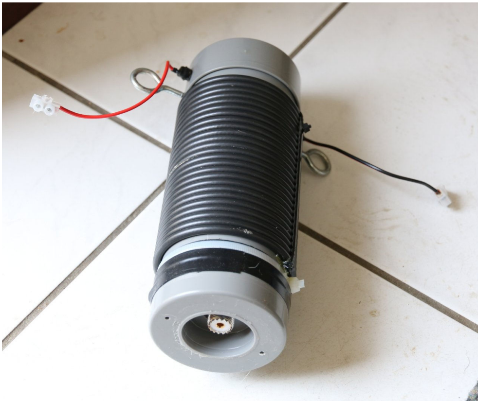
Picture 3 - Ugly balun - Red and black wires connect the dipole with the inner and outer conductors of the coax
