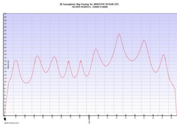
Figure 7 – 3D ray tracing graph, showing a duct between VK7BO to PA2S
