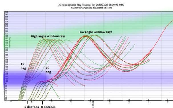
Figure 9 – Ray tracing illustrating the two windows to enter or exit the E-F valley duct.
