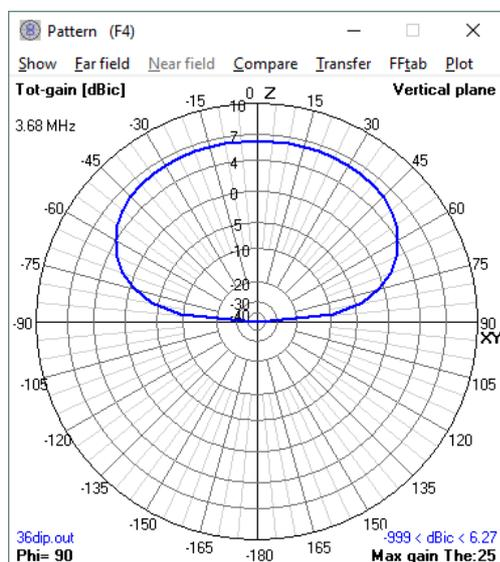
Figure 2 - Theoretical pattern for a low dipole
