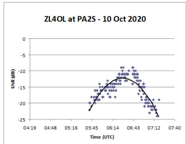
Figure 4 - SNR plotted against time (UTC), ZL4OL to PA2S between 04:30 and 07:30 UTC. The peak around 06:30 is clearly visible.
