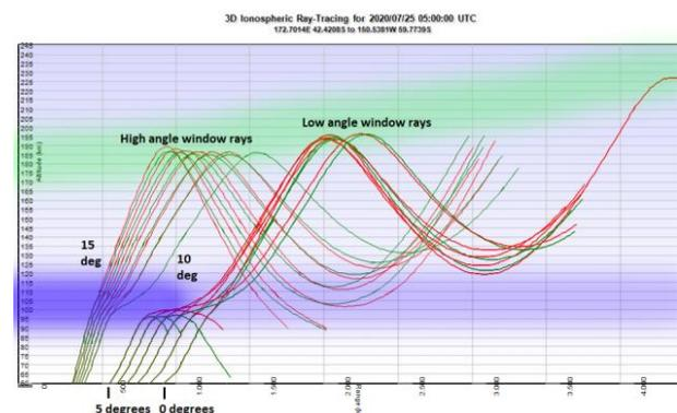
Figure 9 – Ray tracing illustrating the two windows to enter or exit the E-F valley duct.
